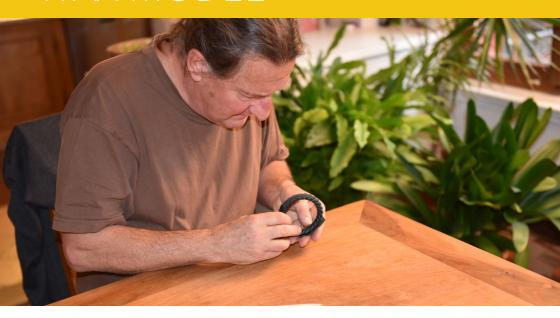
Now the core is completely covered with thin wax platelets. After that, wax sprues are attached by soldering and then joined together to form one somewhat thicker wax sprue.
