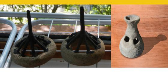
Now the fragile structure is carefully – and in stages – coated with a supporting cloak consisting of fire-proof clay, chamotte and some horse dung. A crucible is formed at the end of the central wax sprue, from which the wax will later flow. The casting mould is dried after each work process.
